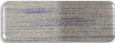
FIGURE [10]SAMPLE [5] USING CREPE STRUCTURE WITH POLYESTER WEFT SLUB
