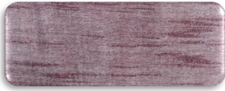
FIGURE [ 8] SAMPLE [3] USING TWILL STRUCTURE WITH BLENDED WEFT SLUB
