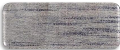
FIGURE [6] SAMPLE [1] USING TWILL STRUCTURE WITH COTTON WEFT SLUB
