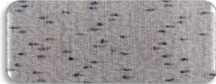
FIGURE [21] SAMPLE [16] USING MATT STRUCTURE WITH COTTON WEFT KNOP
