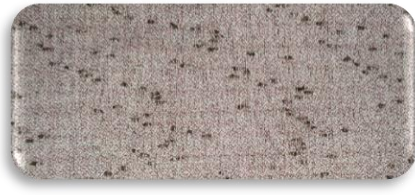
FIGURE [19] SAMPLE [14] USING CREPE STRUCTURE WITH POLYESTER WEFT KNOP
