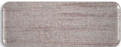
FIGURE [14] SAMPLE [9] USING BASKET STRUCTURE WITH BLENDED WEFT SLUB
