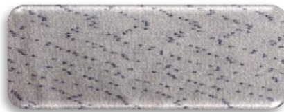
FIGURE [15] SAMPLE [10] USING TWILL STRUCTURE WITH COTTON WEFT KNOP
