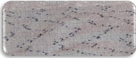
FIGURE [18] SAMPLE [13] USING CREPE STRUCTURE WITH COTTON WEFT KNOP
