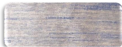
FIGURE [7] SAMPLE [2] USING TWILL STRUCTURE WITH POLYESTER WEFT SLUB
