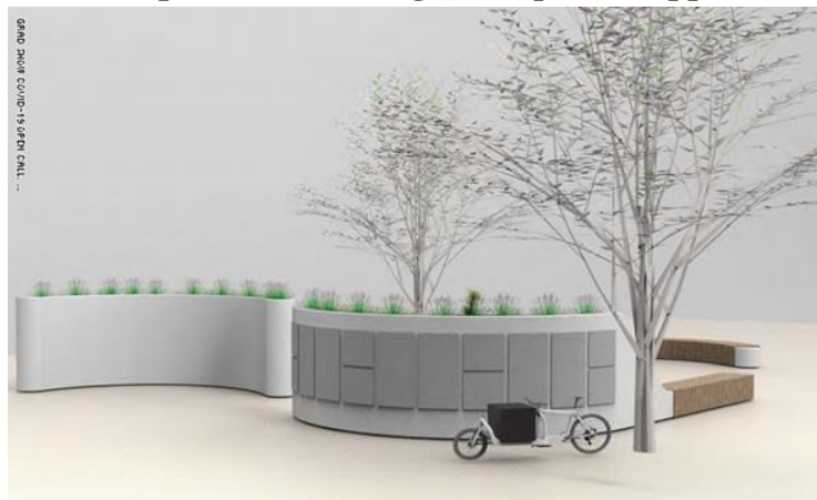
Figure ( 9 ) illustrates the change in the design concept of a supplies receiving space. "Locabox" is a common delivery warehouse where drivers can deliver supplies to multiple addresses simultaneously, and manage their risk of infection. Residents will collect their belongings during specified periods of time.
