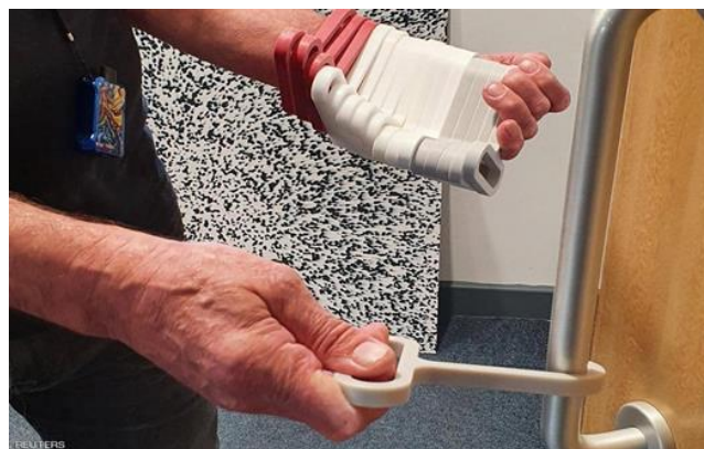
Figure ( 7 ) shows the shape of the sanitary clamp used to handle the doorknobs skynewsarabia.com
