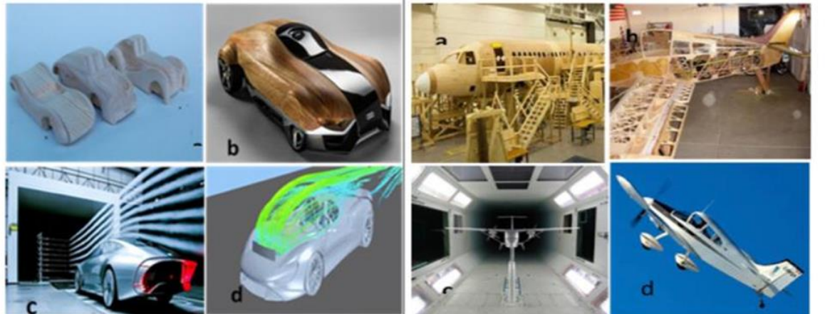
Fig 13: Wood was applied in the manufacture of vehicle models to better comprehend aerodynamics theory. (Jnido,G. et al., 2019)
