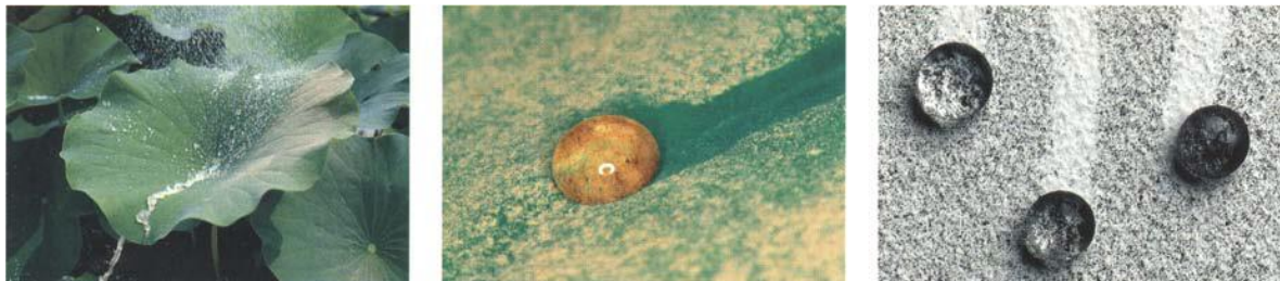
Fig. 6 Lotus plant, a microscopic view of a water droplet resting on a super hydrophobic knobby surface and how the basic principle of the Lotus-Effect works
