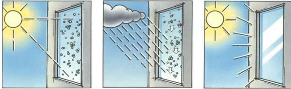
Fig. 9, show organic dirt and grime is broken down and " decomposed". UV light, present in sunlight, is necessary to initiate photocatalysis. When water impacts on the surface, it spreads to form a film washing away the loose dirt. [6].
