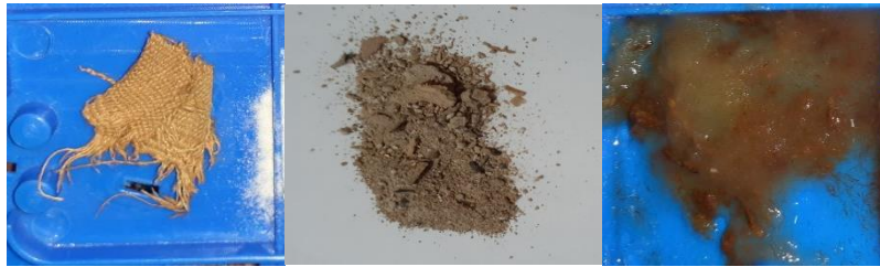
fig 4. Show separated part, after grinding and powder sample with Baraloid B72
