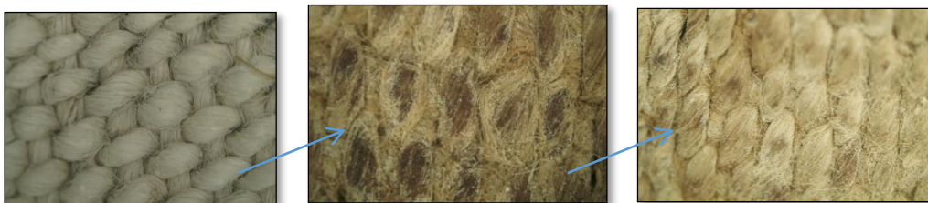
fig.5 microscopic photos show the difference between the new natural linen and the aged one
