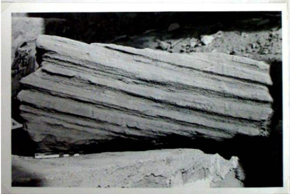
Plate 11 Fragment #657 in an advanced stage of granular disintegration along sedimentary strata, 2001
